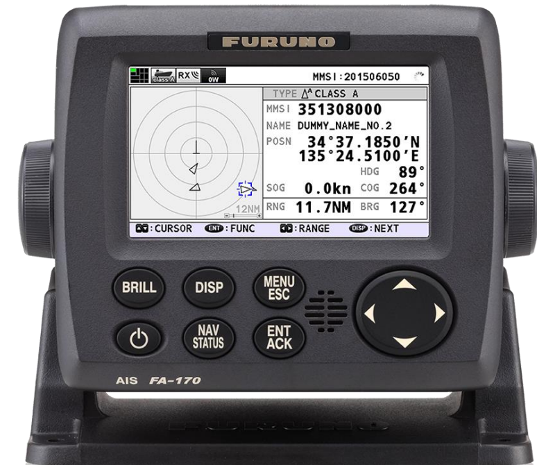
Display unit of a class-A AIS station
