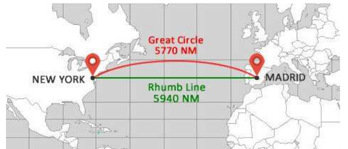
Fig. 5. The great circle path is generally shorter than the direct, or rhumb line, path [31].
